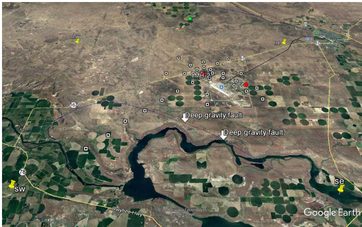
Figure 1: Mountain Home area showing the locations of boreholes MH-1 and MH-2 (red circles) and MT stations (white rectangles). The blue line (indicated by white arrows) passing to the south of MH-1 and MH-2 denotes a deep gravity fault. The NW (Lat: 43.1240, Long: -116.0780), NE (43.1211, -115.7707), SW (42.9439, -116.0807), and SE (42.9411, -115.7743) denote the four corners of the area (25 km by 20 km) used for the numerical model described below.
